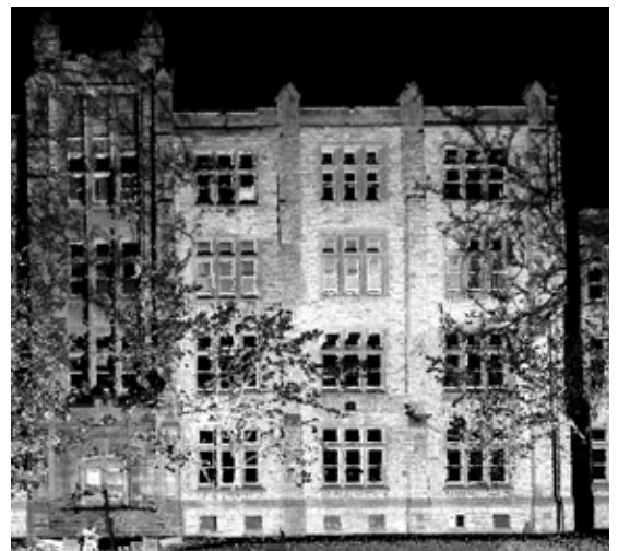
LIDAR model of Miller Hall, Queen's University, collected with an ILRIS time-of-flight LIDAR in October, 2006. It looks like a grainy black and white photograph, but is actually tens of thousands of three dimensional locations, shown here using a software viewer.
