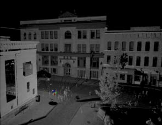
Kingston Whig-Standard building and area point-cloud, scanned November 2007 with a Leica HDS-6000 phase-based, tripod-mounted LIDAR
