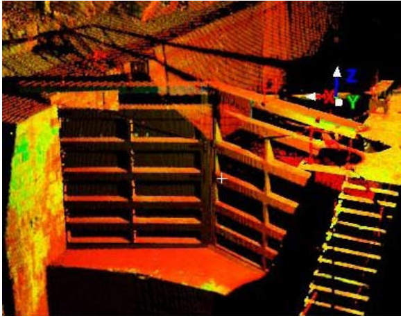
Scan data for the Kingston Mills locks from a Leica HDS6000 ultra-high resolution scanner. The scanner was at the point shown by the x,y,z axes. Scanning the entire region from this point took less than 5 minutes and generated a point cloud of more than 100 million locations. The color indicates the strength of the signal return from the target.
