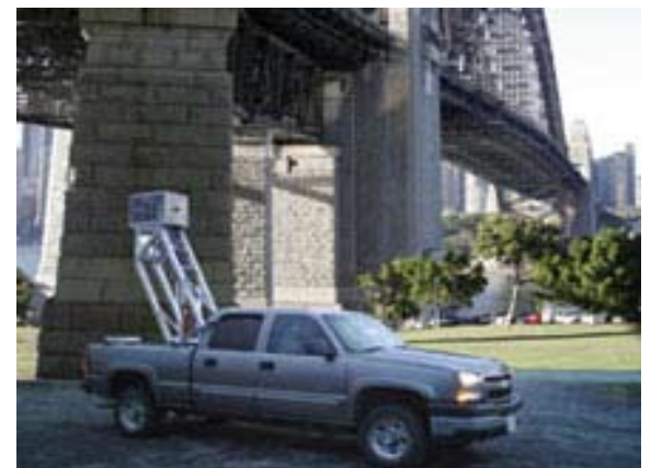
The Terrapoint TITAN scanning solution mounted on a truck. The box mounted on the scissor-lift contains multiple LIDAR and IMU units as well as a GPS receiver. The operator sits in the passenger seat in the truck.
