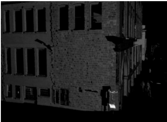
Although this resembles a LIDAR point cloud, this is a surface representation of the edge of the Kingston Whig Standard building constructed using surfacing tools in Leica's CYCLONE LIDAR processing package.
